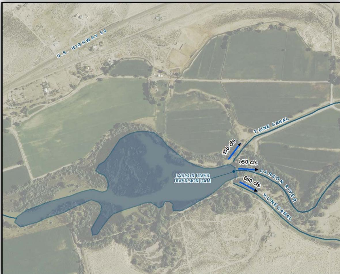
**Figure 3 – Existing Flow Diversion Plan at Carson River Diversion Dam**
