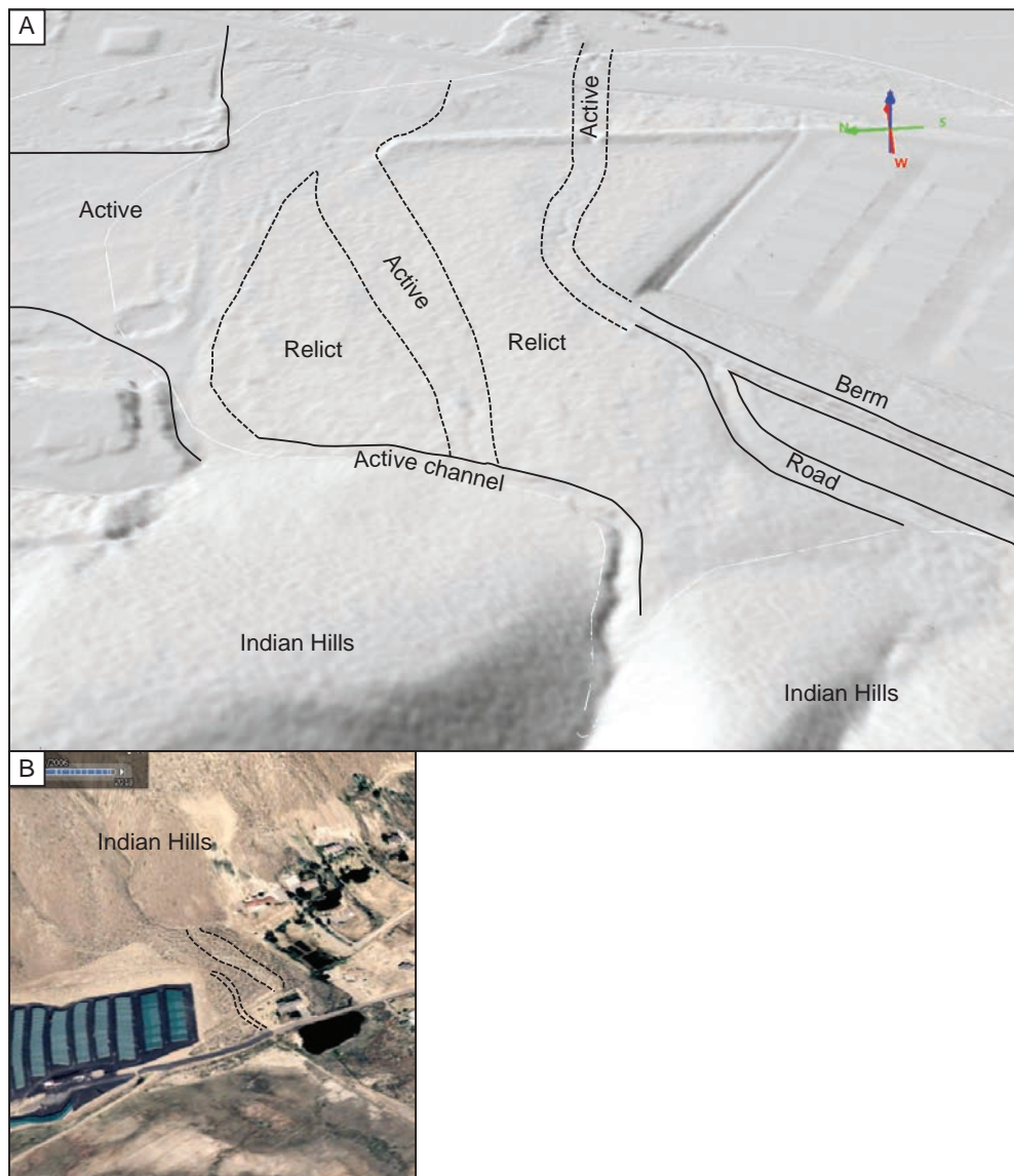
Figure 19. Evidence of recent alluvial activity on Fan 81. A) Oblique view looking to the north of a hillshaded relief model. There are two zones (marked active in center of image) where there has been channelization caused by surface flow. The GoogleEarth aerial photograph shown in B) was taken in October 2006. Approximate area of the active zones highlighted in A) are dashed. Fan 82
