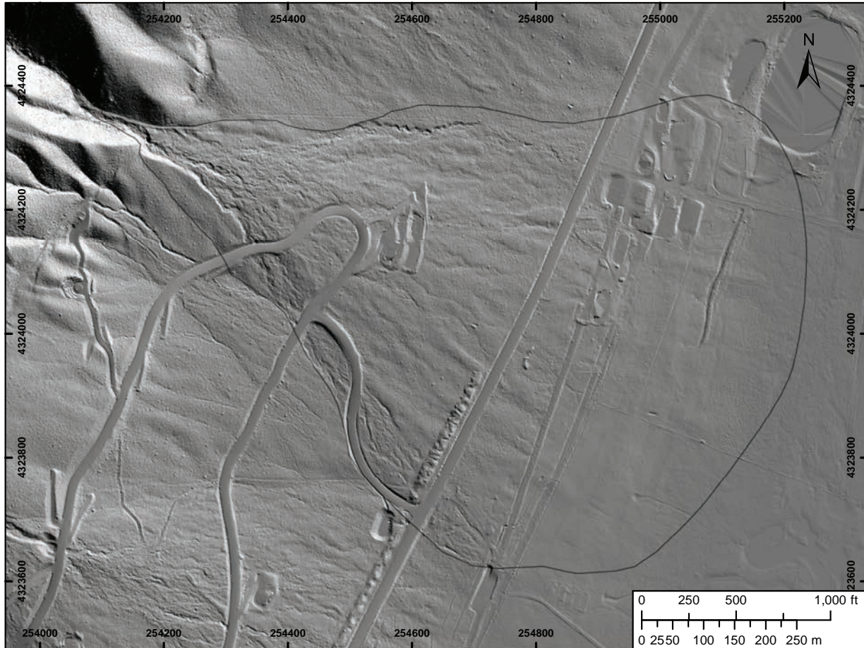
Figure 38. Fan 45. Shaded relief hillshade image made using 2017 LiDAR data imported at a cell resolution of 0.29 m (0.95 ft) using the software Quick Terrain Modeler. Illumination is from the north to accentuate channels on the alluvial fan surface. Note fine, branching nature of channels on the northern half of the fan and along the southern fan boundary. Flat, semi-rectangular pads represent building foundations.
