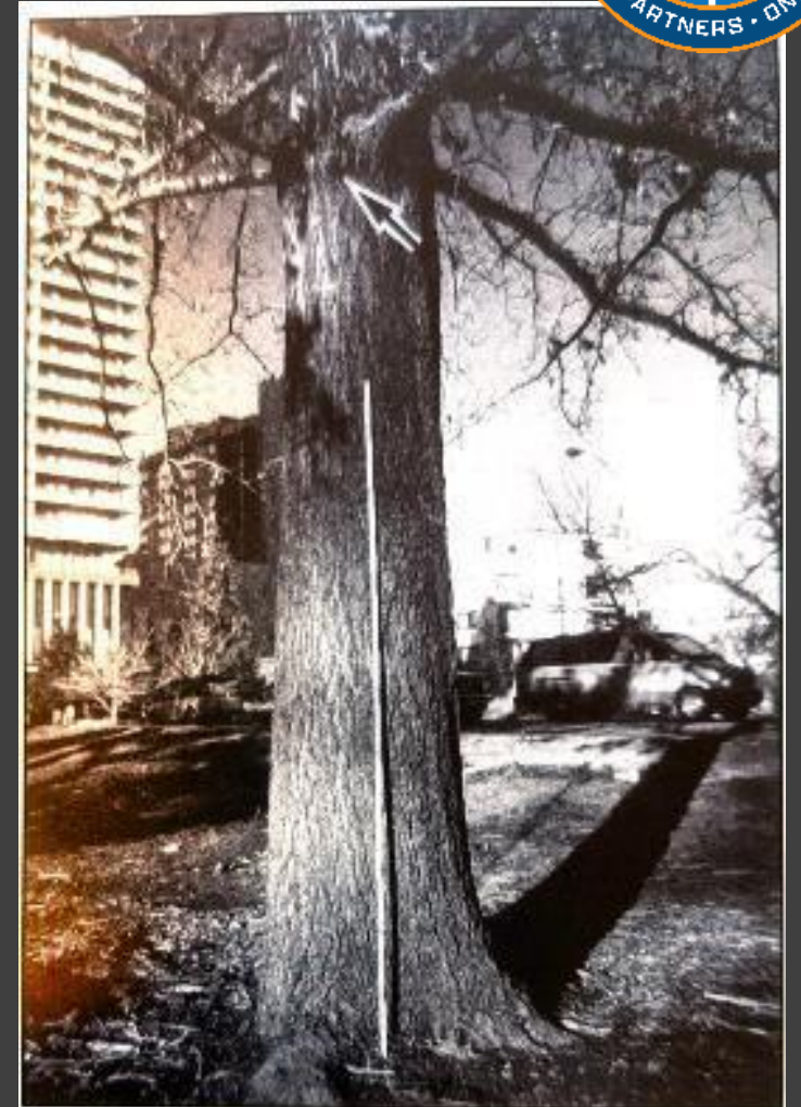
Photo 12 — Measurement of high-water mark on tree in Wingfield Park just west of Arlington Avenue
